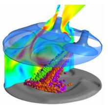
View larger image P Automotive in-cylinder flow model with ANSYS CFX Software (Courtesy of BMW)
